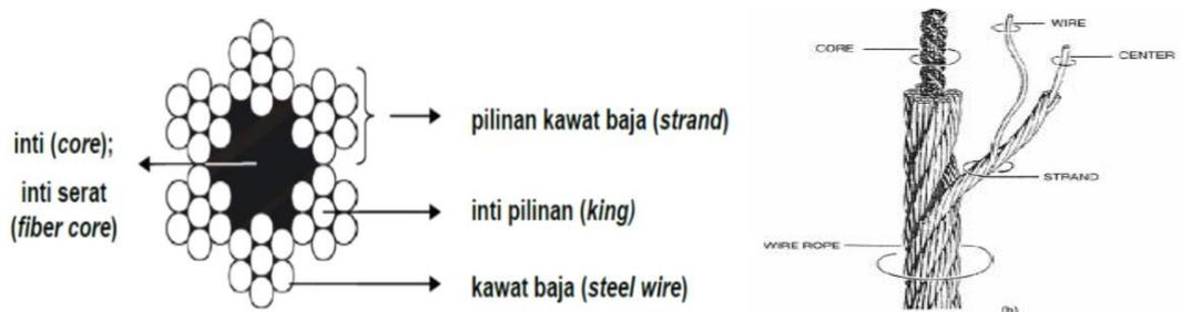
**Gambar 1.** Tipikal Geometrik *Wireropedapat* (SNI 0076, 2008)
