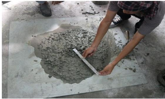
**Gambar 3.** Hasil pengujian *slump flow spread*
