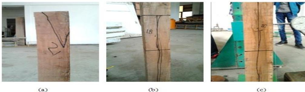
Gambar 10 Pola keruntuhan (a) KH1 (b) KH2 (c) KH3
